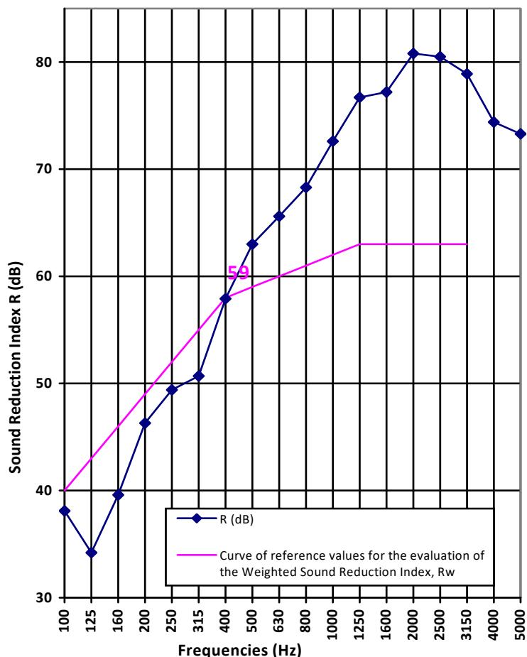
Rating according to EN ISO 717-1:2013: R<sub>w</sub> (C;C<sub>tr</sub>): 59 (-3; -8) dB
