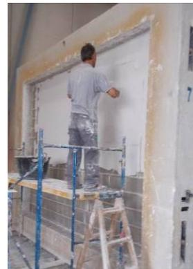
Block: 500 mm long x 190 mm high x 150 mm thick & 14,2 kg (estimated superficial mass: 149 kg/m<sup>2</sup>).
